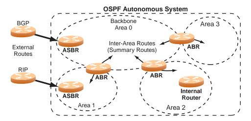
Figure 4-2 OSPF Domain and an Autonomous System
